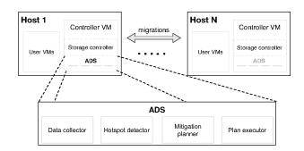
Figure 4: ADS high-level design
