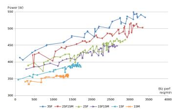
Figure 7: Business Performance (Req/min) versus Power Consumption (W) for each working mode
