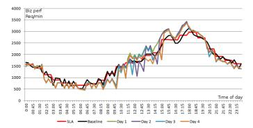
Figure 6: SLA and measured performance for each day
