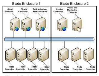
Figure 4. The logical view of the main hardware resources.
