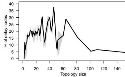
Fig. 6. Percent of delay nodes per experiment
